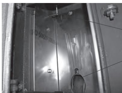
Fig. 133 Cleaning the thermocontrol sensor (with cleaning brush) and down chute
