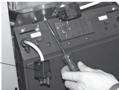
Fig. 155 Removing the power plug and screw
