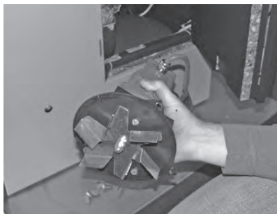
Fig. 162 Cleaning the blower wheel
