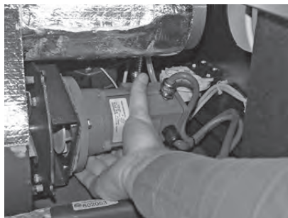
Fig. 161 Removing wing nuts, removing the blower unit
