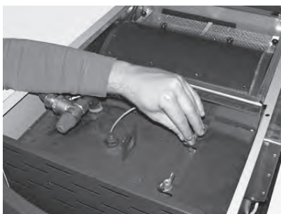
Fig. 149 Removing the wing nuts and cover
