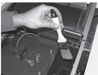
Fig. 151 Cleaning top heating surfaces and linkage
