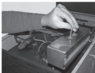
Fig. 150 Removing the jet protection plate
