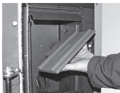
Fig. 132 Removing and cleaning the baffle plate
