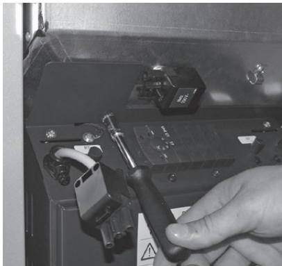
Fig. 46 Disconnecting the mains power plug and removing the screw.
