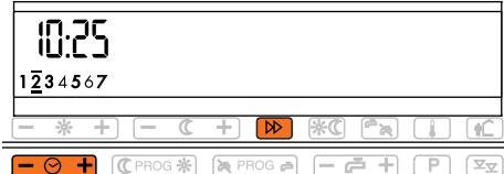
The display returns to normal after 1 minute, or you can press the
